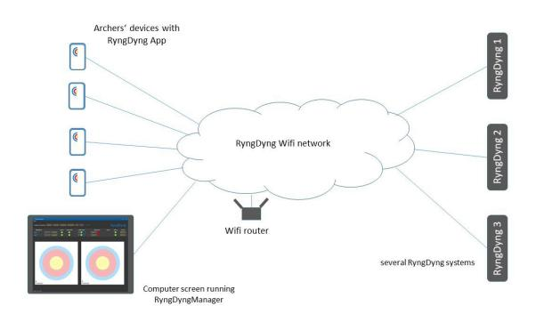
It is also possible to connect the RyngDyng systems to an Ethernet switch, which then connects to the Wi-Fi router LAN port. This way it is possible to use the Wake-on-LAN feature supported by the RD720 devices.
